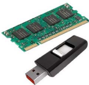
Fig. 1: DRAM and Flash memories (USB-Stick)
